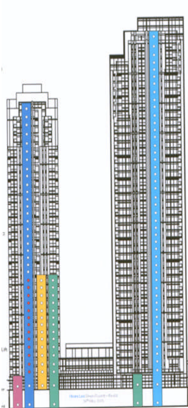
Figure 14 – Lift layout for high-rise building
